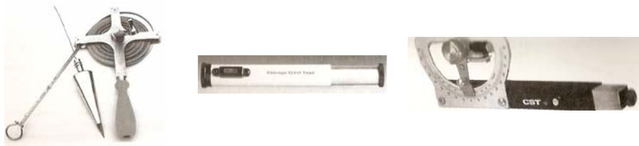
(steel tape, hand-level and clinometer)
