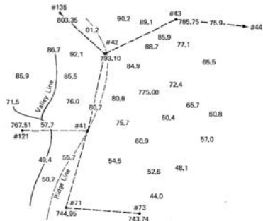
FIGURE 8.6 Plot of survey control, ridge and valley lines, and spot elevations.
